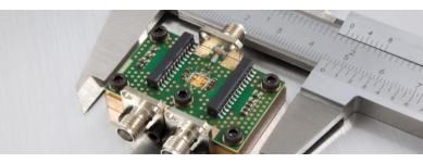
Fully digital transmitter chain for base station application.
